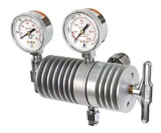
The SR311-320 CO2 Flowmeter adjustable pressure gauge is specifically designed for use with standard (non-siphoned) carbon dioxide cylinders. Our unique design incorporates aluminum heat sink fins which permit high flow rates without freeze-up.
