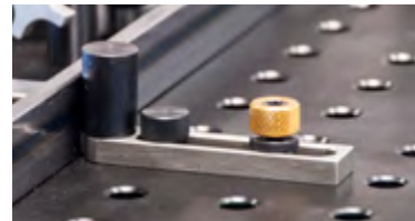
The spring loaded pin provides variable pressure for the quick locating, placement and removal of stock.
