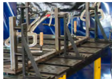
Insert V-Blocks to support round stock.
