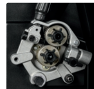
Heavy-duty aluminum two-drive-roll system
