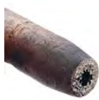
Nozzle fully clogged (not using E-WELD Nozzle)
